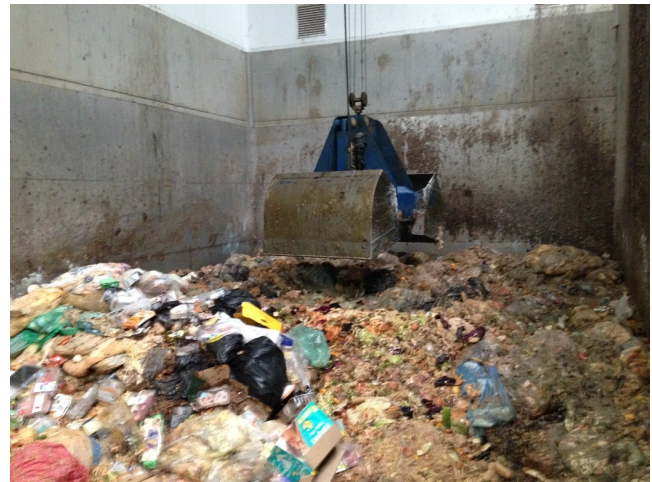
Figure 3.2: Clamshell grab at a food waste AD
