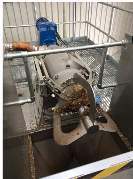
Figure 6.2: Example of a screw press digestate separator
